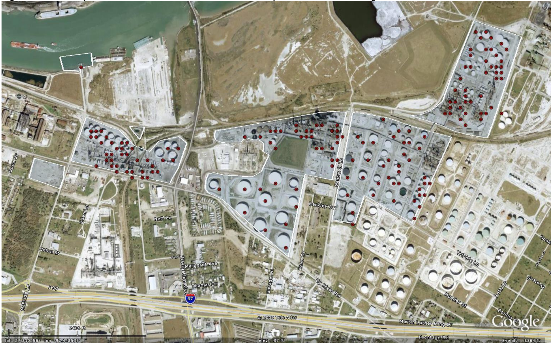
Figure 10. Emission points for the Valero East site in the 2005 TCEQ Photochemical Modeling EI.
