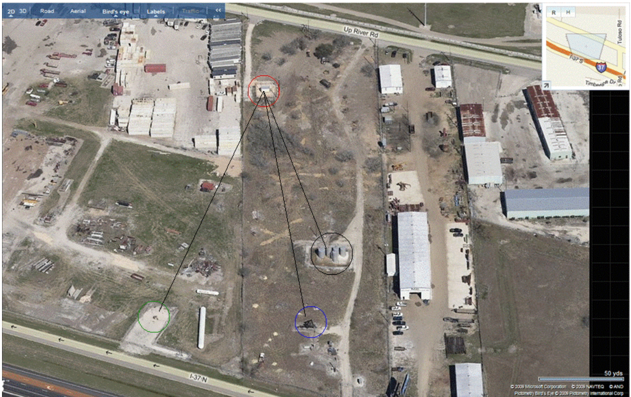
Figure 21. Red circle is CAMS 632, black circle is tank battery 150 meters away at 164 deg. from north, blue circle is pump jack 200 meters away at 172 deg., green circle pump jack is 197 meters away at 193 deg. Tank battery on south side of IH37 from Figure 20 is 390 meters away at 184 deg.
