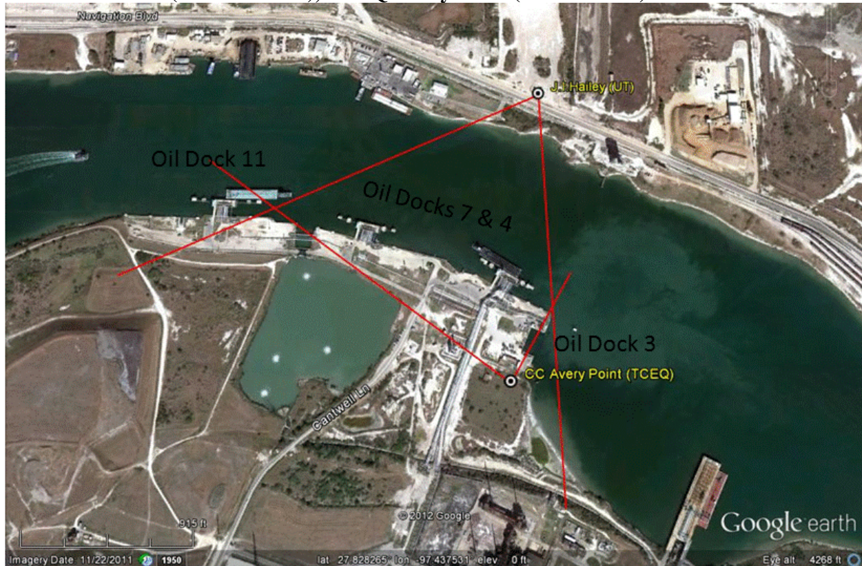
Figure 15. Rays drawn in key directions associated with highest SO 2 concentrations at two CAMS sites: JIH (178° and 246°), TCEQ Avery Point (30° and 306°)
