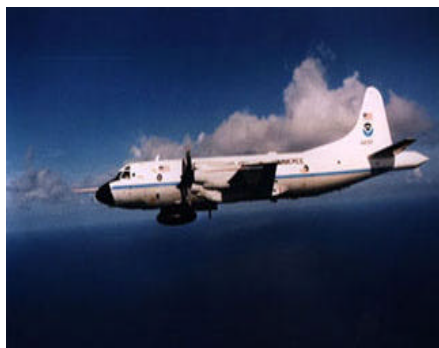
Lockheed WP-3D Orion: NOAA Aircraft Operations Center / NOAA Aeronomy Laboratory Endurance: 10 hrs; Ceiling: 7.6 km; Payload: >2700 kg; Research Speed: 100-150 m/s
