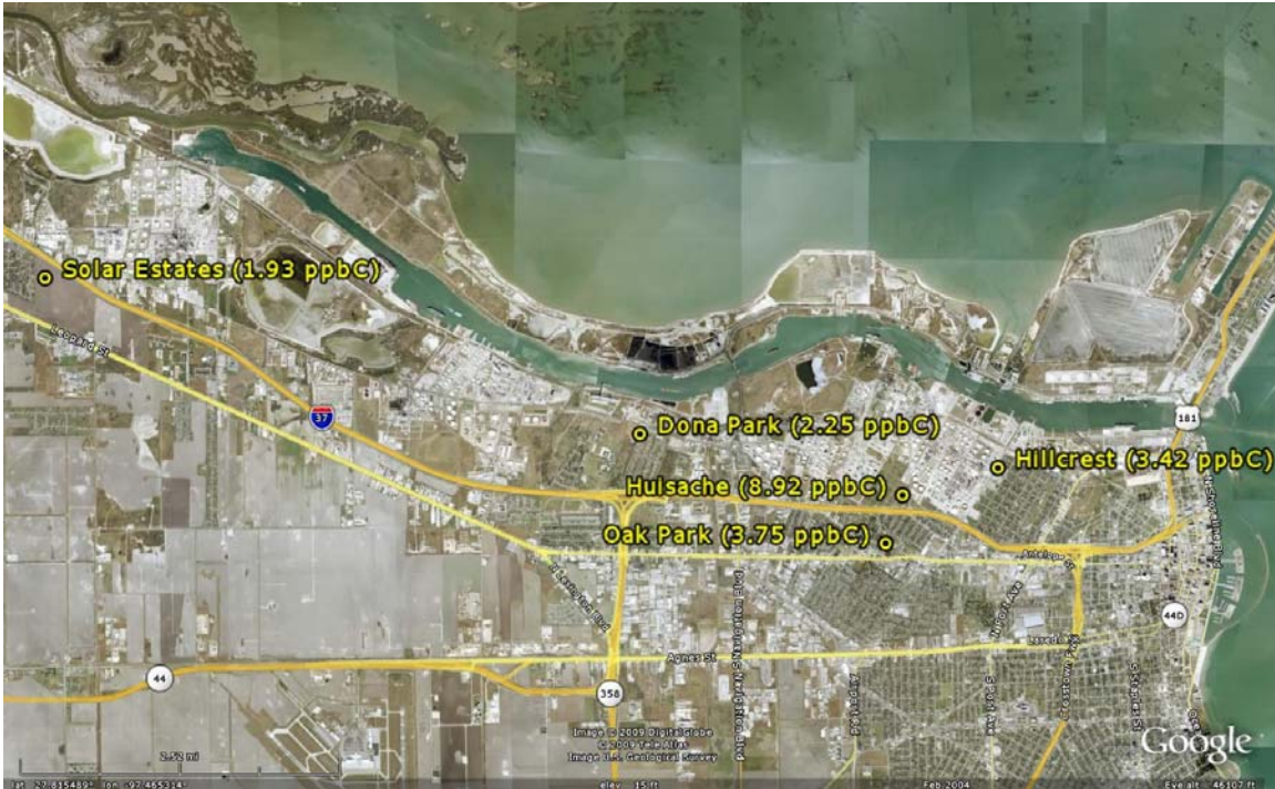
Figure ES-3. Average benzene concentrations during June 2005 – May 2008 at (1) CCAQP Oak Park and Solar Estates monitoring stations using hourly measurements, and (2) Corpus Christi CATMN stations using 24-hour sampling measurements.
