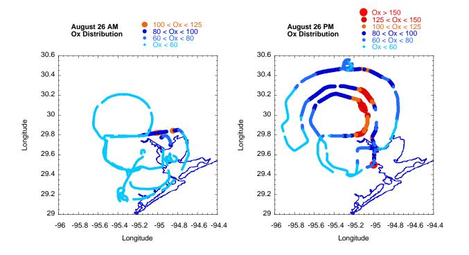
AM-Background  $O_3$  concentrations ~ 30 - 40 ppb. Observed small  $O_3$  plume NE of ship channel late in flight.
